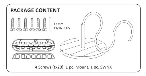
Mounting requires additional tools: 1 pencil + screwdriver. Attention: Table thickness should be over 20 mm (13/16 in US)
